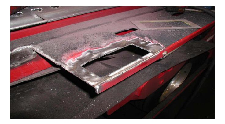
STEP 6: INSTALL NEW COVER PLATE OVER HOLE IN CATWALK. WELD 50%
