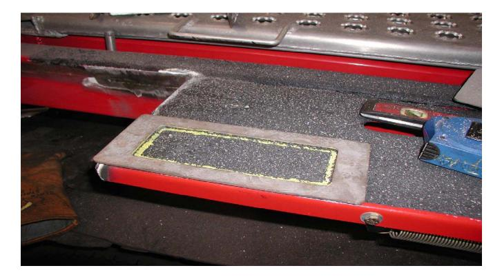
STEP 5: CUT OUT HOLE AND GRIND SMOOTH.
