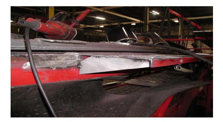
STEP 5: PLACE TEMPLET ON THE OUTSIDE CORNER OF THE CATWALK AND MARK HOLE.
