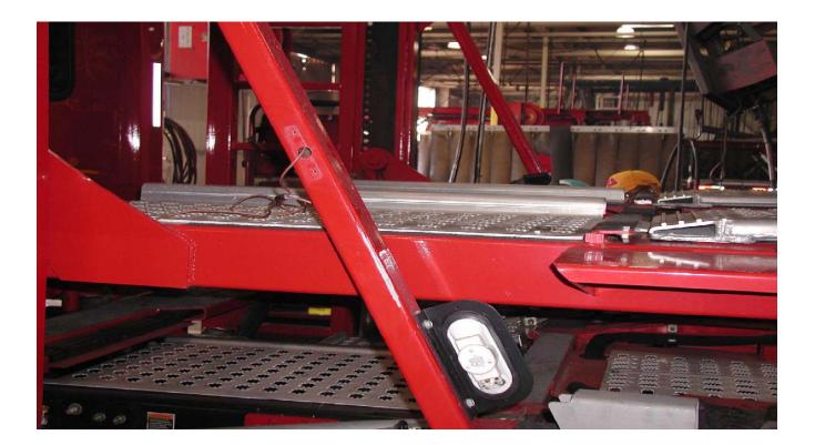
STEP 2: INSTALL GRAB HANDLE BRACKET FLUSH WITH CATWALK ON RUT
